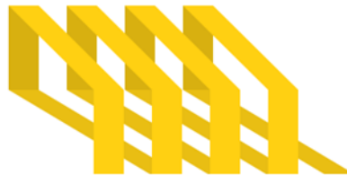
Figure 1.5: Example of a solenoid of rectangular geometry
